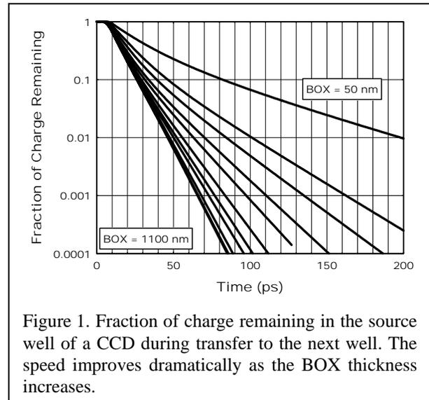
Figure 1. Fraction of charge remaining in the source well of a CCD during transfer to the next well. The speed improves dramatically as the BOX thickness increases.
