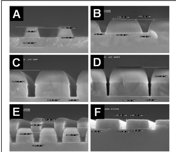
Figure 2. Series of SEM images showing the steps in the fabrication of narrow gaps within a single layer of polysilicon gate material.
