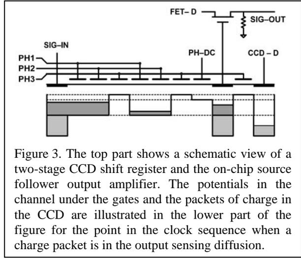
Figure 3. The top part shows a schematic view of a two-stage CCD shift register and the on-chip source follower output amplifier. The potentials in the channel under the gates and the packets of charge in the CCD are illustrated in the lower part of the figure for the point in the clock sequence when a charge packet is in the output sensing diffusion.
