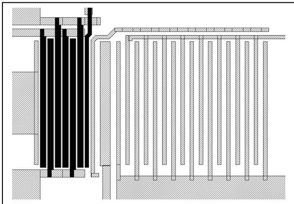
Figure 4. This is a captured image of the layout of a two-stage CCD, corresponding to the diagram in Fig. 3. The polysilicon gates are shown in solid black on the left. Metal wiring is shown in grey. The structure on the right is the large, interdigitated FET of the output amplifier. Only the metal lines that contact the source and drain are shown; its polysilicon gates, which are defined in a different drawing layer, have been suppressed.
