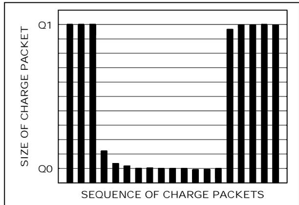
Figure 5. Sequence of charge packets read out from a 200-stage CCD shift register. The input packets formed a square pulse with small packets ( $Q_0$ ) and large packets ( $Q_1$ ). The rounding at the transitions is the result of imperfect charge transfer, estimated to be about 0.9995 per stage or 0.9998 per transfer.
