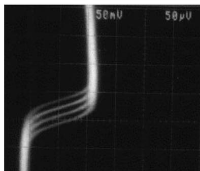
Fig. 10. Oscilloscope photograph showing a superposition of numerous outputs from the dc SQUID monitoring the samples stored in the T/H cell. The quantization of the stored samples can be seen clearly.
