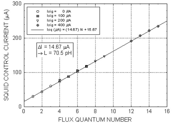
Fig. 11. Plot showing the current in the control line of the dc SQUID output detector corresponding to a range of quantum states in the T/H cell. The total inductance in the sampler storage loop can be determined accurately from the size of the quantum step in current.
