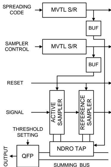
Fig. 2. Detailed block diagram of one slice of the filter along with the output detector circuitry.
