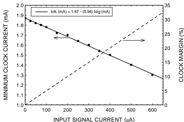
Fig. 9. Clock margins for the buffer between the digital shift registers and the analog components. The points are measured data. The solid curve is a least-squares fit to a straight line, with the equation shown in the legend.
