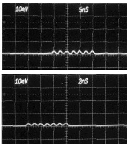
Fig. 8. These oscilloscope photos show the output from the MVTL shift register in the complete seven-stage filter. The clock frequencies were 400 MHz for the top photo and 1 GHz for the bottom photo.
