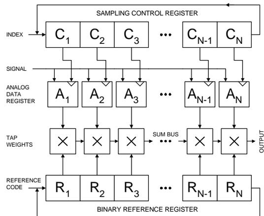
Fig. 1. Block diagram of the superconductive programmable matched filter.
