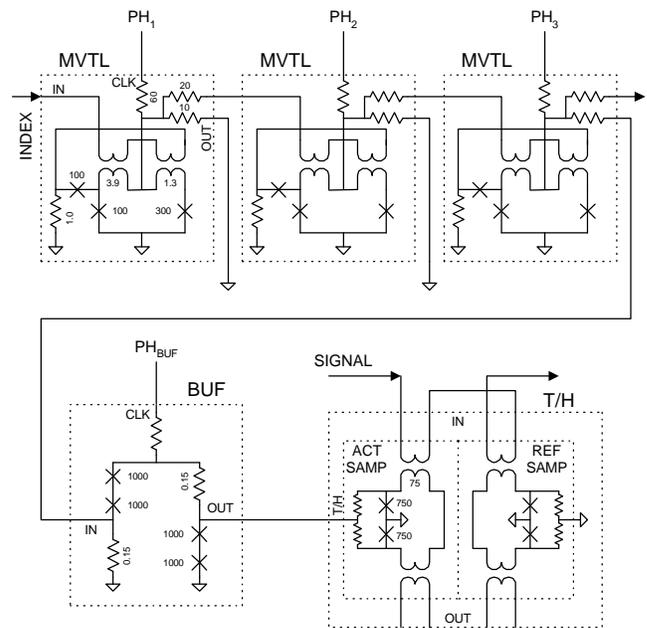
Fig. 3. Circuit schematic of the T/H channel of the filter, including the MVTL shift register, the buffer, and the T/H circuit. The component values shown are nominal values, and damping resistors across the junctions are not shown. Resistances are in ohms, junction critical currents in microamperes, and inductances in picohenries.
