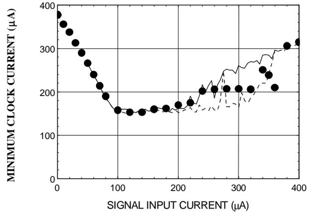
Fig. 6. Clock margins for a loaded OR gate in a shift register. The points are measured values. The dashed, lower curve is the lowest clock voltage at which a JSIM simulation showed the gate switching, while the solid, upper curve shows the lowest clock voltage for which a JSIM simulation showed the gate not switching. Between the two curves simulations sometimes showed the gate switching and sometimes not.
