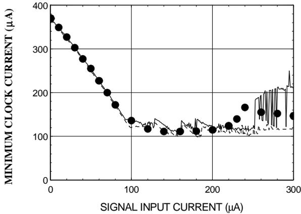
Fig. 5. Clock margin for an isolated MVTL OR gate. The points are measured values. The solid curve was calculated using the JSIM simulator with a simulation interval of 10 ns, while the dashed curve was for a simulation interval of 50 ns.
