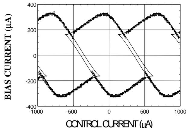
Fig. 4. Experimental MVTL SQUID characteristic (points) with overlay of best theoretical fit (solid curves). The bias current corresponds to the clock current of the MVTL gate, while the control current corresponds to the input signal current.
