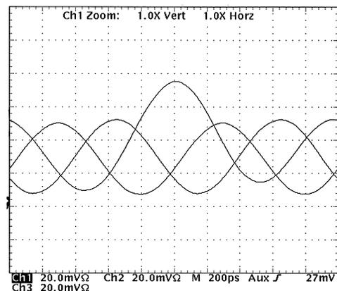
Fig. 7. Traces from a digital real-time oscilloscope showing the three-phase sine-wave clocks with the extra offset added during one cycle.
